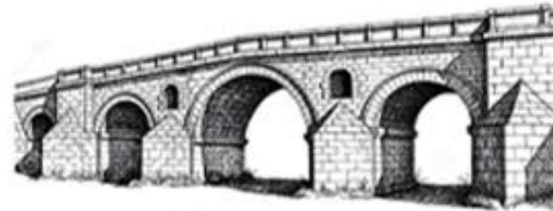
Deck Arch Bridge
