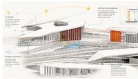
Vertical breakers on the west front
