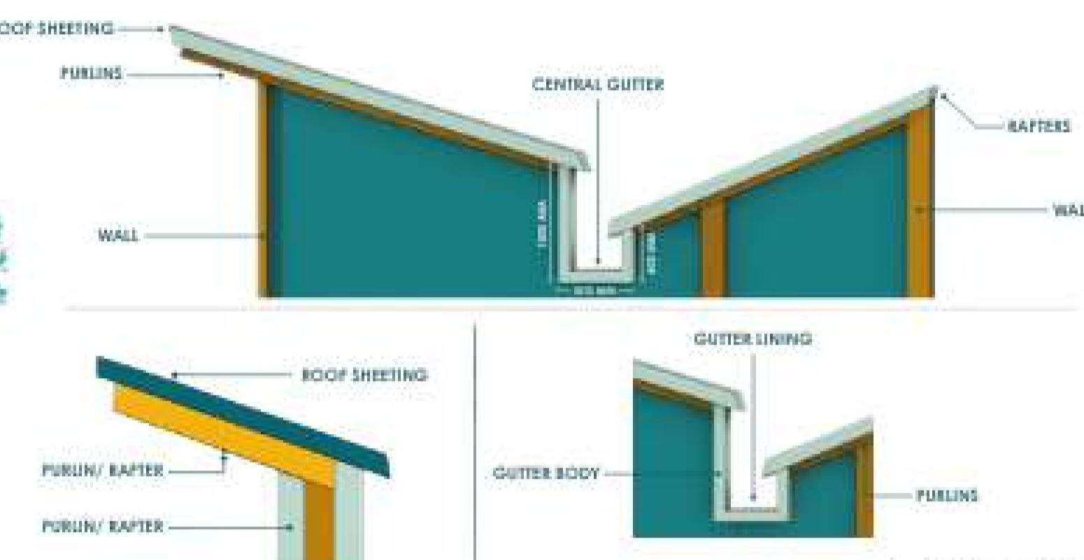
Detail at 'H' (Butterfly roof)
