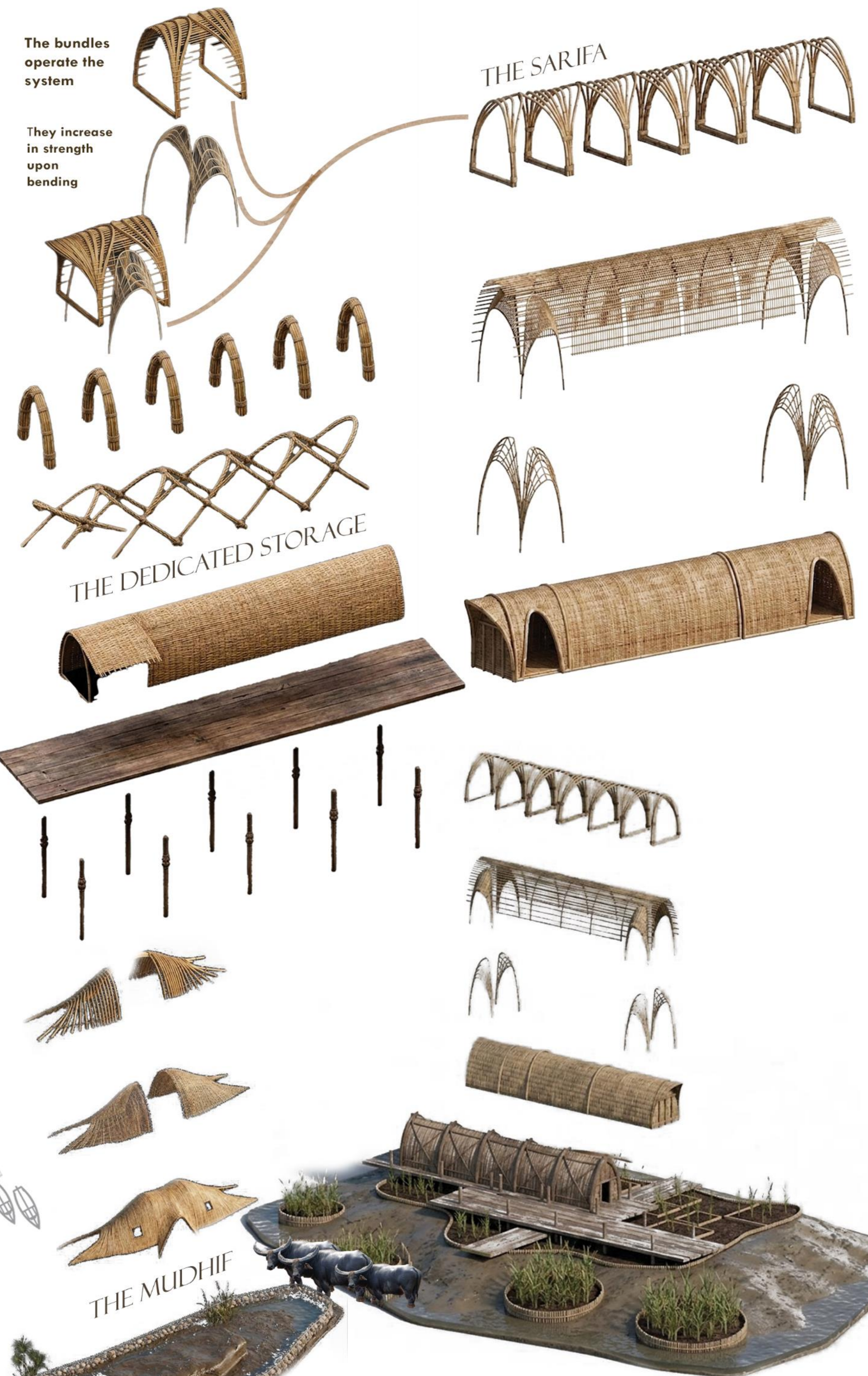
Massive reed bundles (40–80 cm in diameter) are anchored deep into the marsh soil at an outward angle. Opposing bundles are then pulled together and interwoven.
