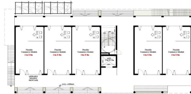
GROUND FLOOR PLAN OF NEWLY DESIGNED MODULE, TYPE 2
