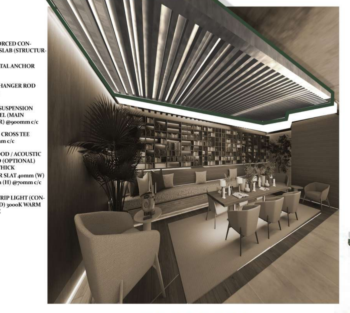
TIMBER SLATTED CEILING DETAIL
