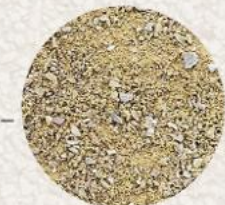
CRUSHED STONE WALKABLE SURFACE
