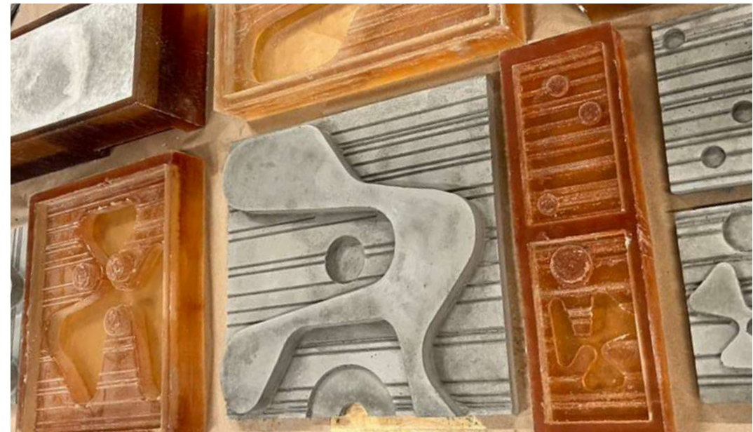
Figure 32: Molds and tiles after demolding and be cured.
