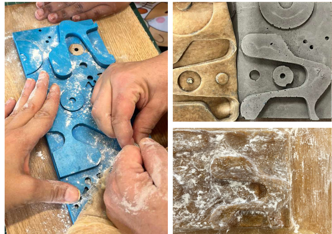
Figure 28: Photos of demolding latex from cardboard with baby powder and demolding the concrete cast.
