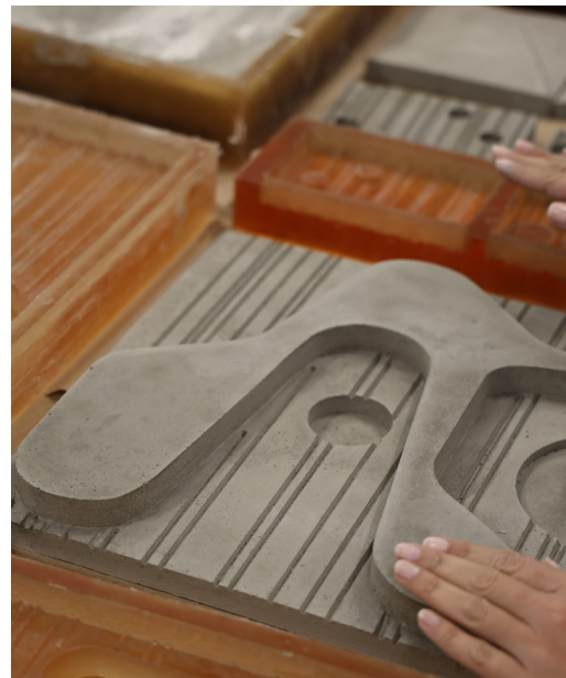
Figure 30: Mold and concrete tile.
