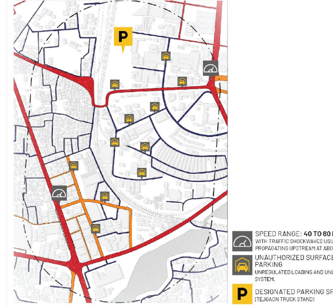
FIG 06 STREET TYPOLOGY PRIMARY CONNECTION SECONDARY CONNECTION TARTIARY CONNECTION SPEED RANGE: 40 TO 80 KM WITH TRAFFIC SHOCKWAVES USUAL PROPAGATING UPSTREAM AT ABOUT UNAUTHORIZED SURFACE PARKING UNREGULATED LOADING AND UNLOAD SYSTEM, DESIGNATED PARKING SPOT (TEJGAON TRUCK STAND)
