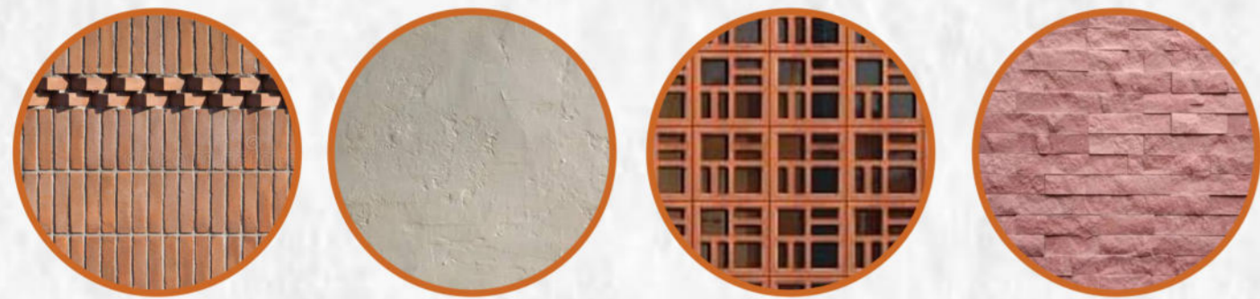
Brick walls Lime plaster Terracotta jaali Pink sandstone
