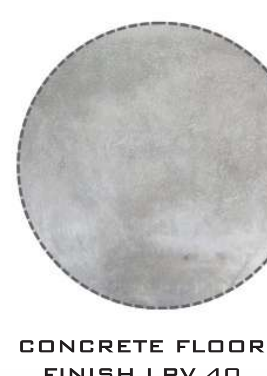
CONCRETE FLOOR FINISH LRV 40
