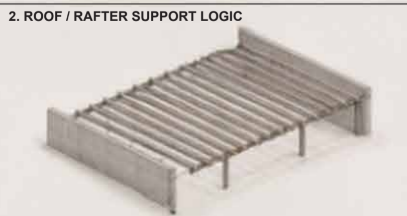
2. ROOF / RAFTER SUPPORT LOGIC Secondary rafters sit on the primary beams, supporting the roof slab and distributing loads while defining the gentle roof slope towards the landscape.
