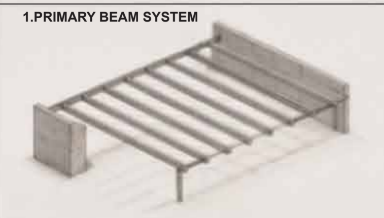
1. PRIMARY BEAM SYSTEM Long span reinforced concrete beams create the primary structure direction, bridging between retaining walls and expressing the pavilion inquarity .
