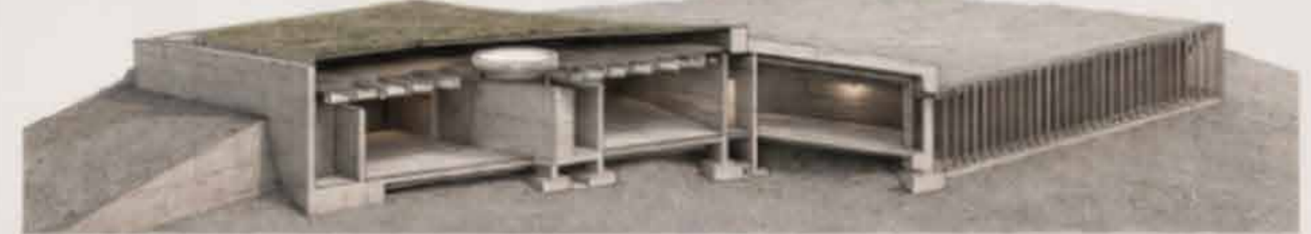
The pavilion is held between retaining walls, with beams spanning across to create an open interior volume. The structure works with the landform, establishing a continuous journey from earth to light.
