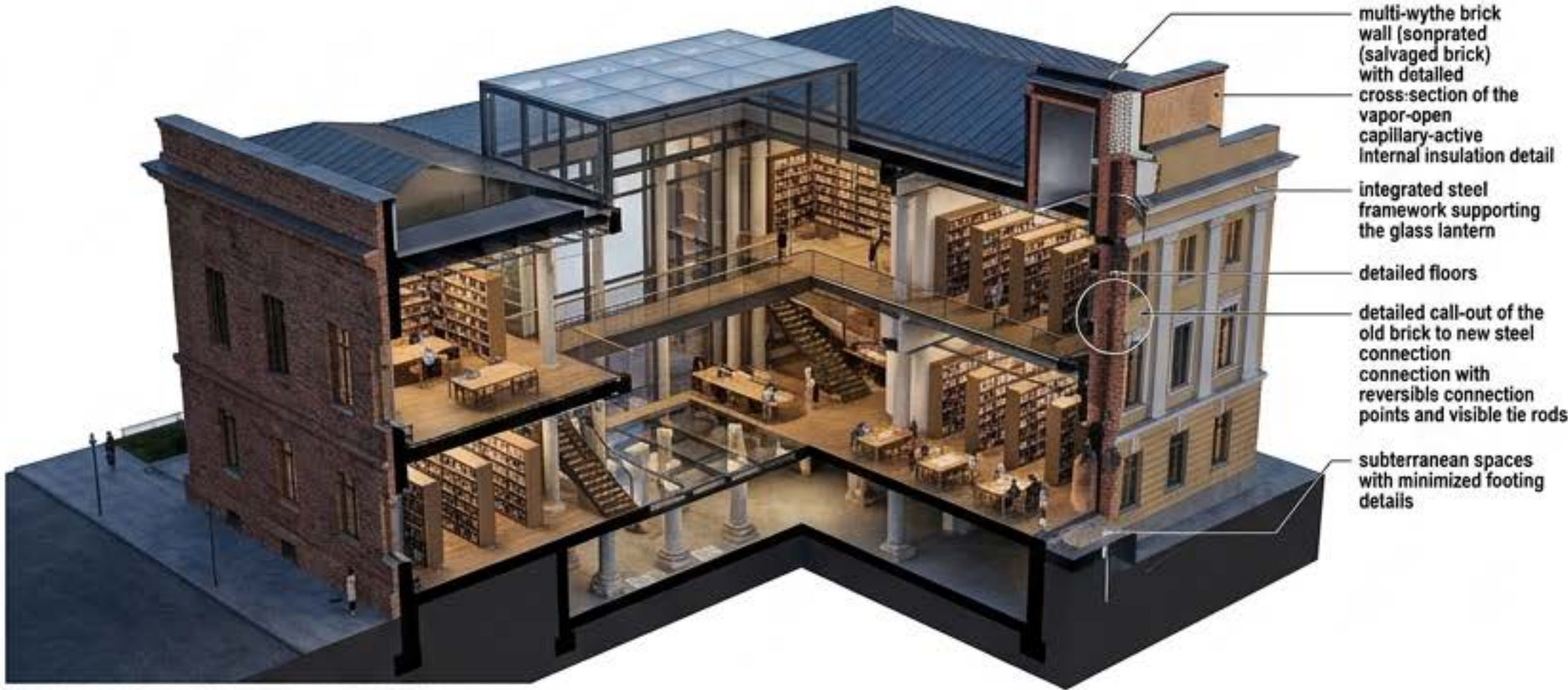
SPATIAL THEORY: INTEGRATED HYBRID SECTION narrative transparency, structural reversibility, thermal comfort detail
