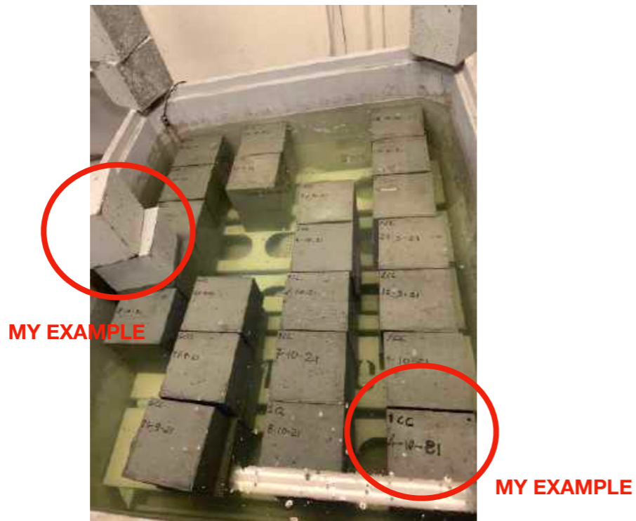
CHECKING THE STRENGTH OF CONCRETE IN WATER +10 DEGREES
