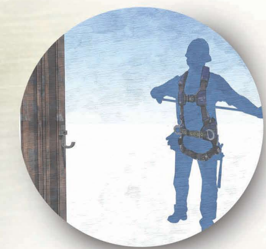
HARNESS FIXATION ON THE RAIL COLOUMNS TO HOOK WHILE MAINTENANCE
