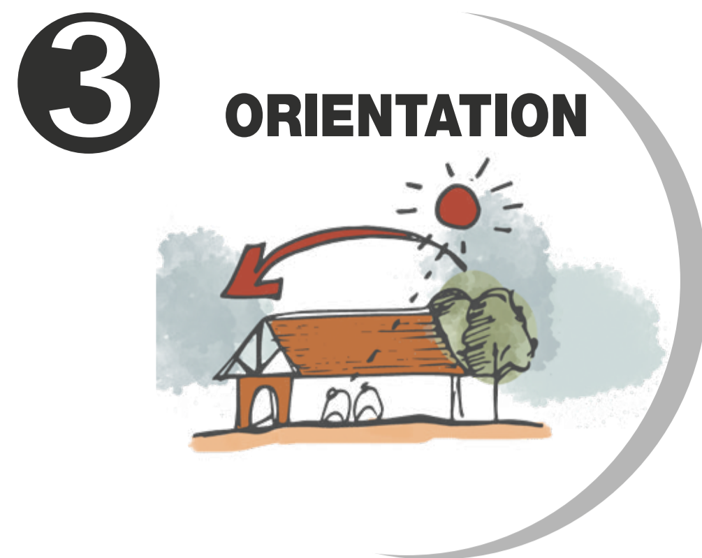
3 ORIENTATION ALIGN SHORTER FAÇADE TOWARD EAST-WEST AXIS; REDUCING EXPOSURE TO SOLAR RADIATION FOR ENCLOSE HABITATION
