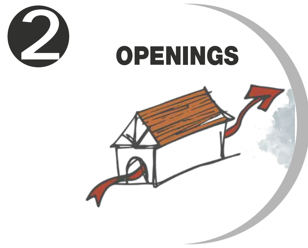
2 OPENINGS MORE OPENINGS ON NORTH - EAST AND SOUTH WEST FACING FAÇADE TO ALLOW PREVAILING WINDS TO VENTILATE THE SPACES OF HABITAT AND FACILITIES BUILDINGS
