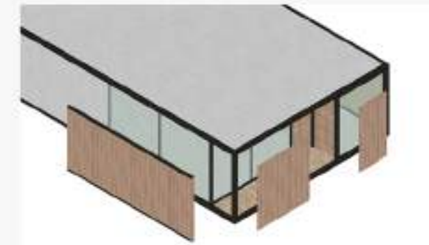
ADAPTABLE FACADE WITH MOVABLE WOOD PANELS
