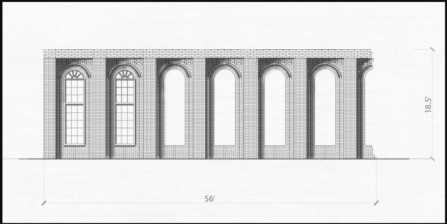
Courtyard North Elevation
