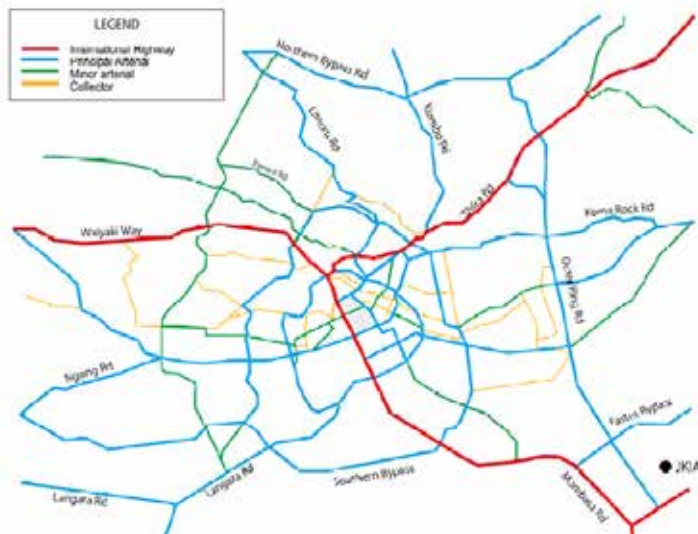
Photo Excerpt from the New Integrated Urban Development Plan Showing Classification of Future Road Network 2030
